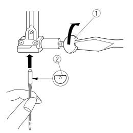
Insert a new needle into the needle clamp with the flat side of the needle to the rear.
