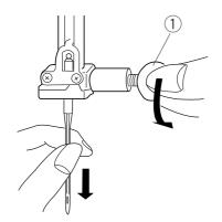
Turn off the power switch. Raise the needle by turning the handwheel and lower the presser foot. Loosen the needle clamp screw by turning it counterclockwise.
